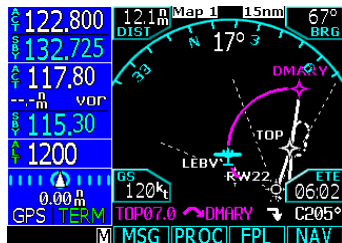
DME Arc Leg shown on moving map and in the course direction description line at the bottom of the screen.
